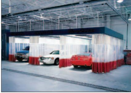
Features a 52" high clear vinyl center section that starts 30" up from the floor. The top section will vary according to your height requirements. Each partition is furnished with two, 2" wide x 1' long Velcro® strips on each side to provide easy access and yet assure a tight seal. A zinc plated chain is installed in the bottom hem. Opaque vinyl panels are available in white, yellow, blue, green, red, gray or black.
